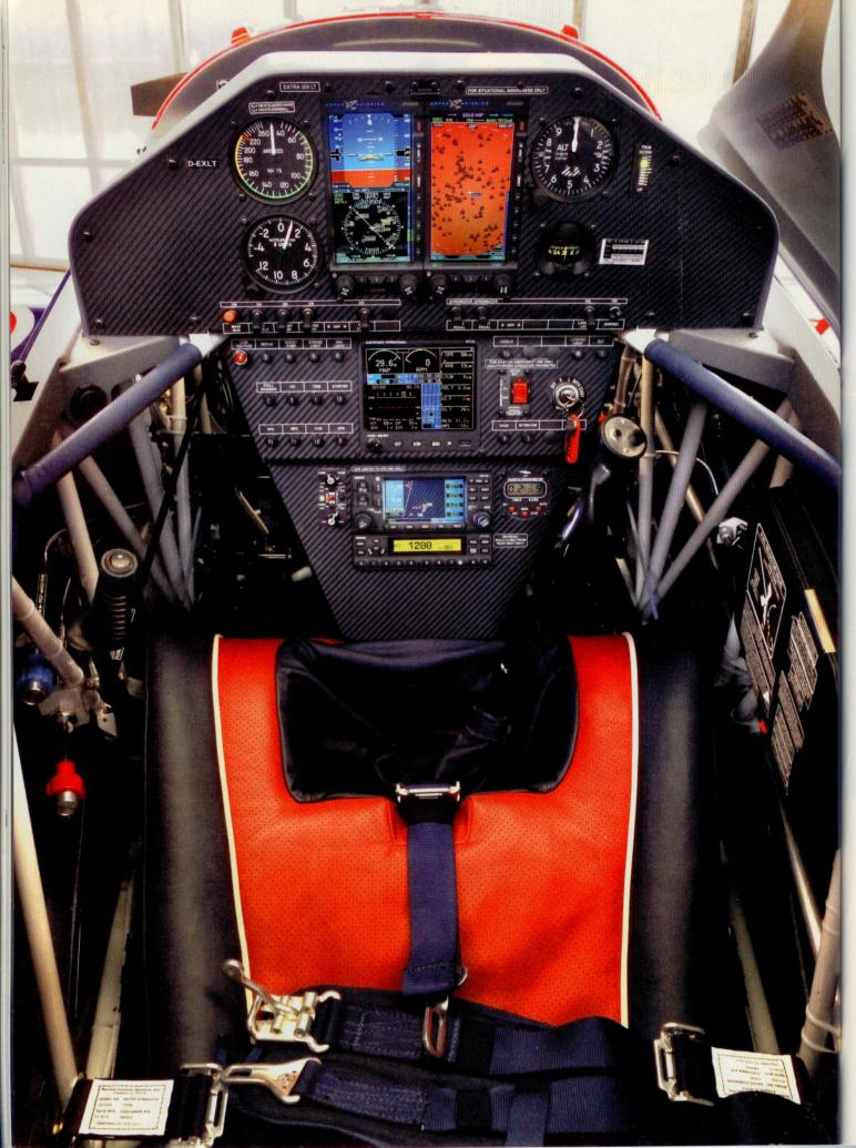
The Extra 330 LT has a two-screen Aspen PFD/MFD in the rear cockpit (left) linked to a Garmin GNS430W. The PFD is designed not to tumble during aerobatics and aggressive maneuvering and can reorient itself in flight. The stick is equipped with a push-to-talk button and an elevator trim switch. A landing light is mounted in the lower cowl and strobes are on the curved wing tips (below). A baggage door accessible from outside the airplane (bottom) is a new addition on the LT.
