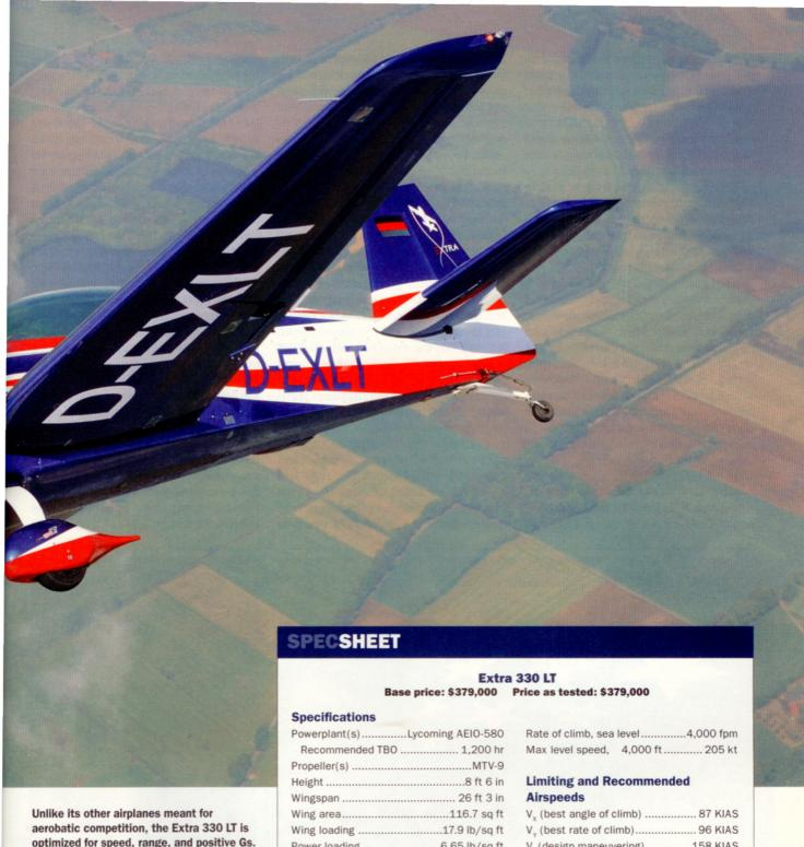
Unlike its other airplanes meant for aerobatic competition, the Extra 330 LT is optimized for speed, range, and positive Gs. The non-symmetrical airfoil is identical to a racer Extra designed and built for the Red Bull pylon racing series. The LT prototype, shown here in the skies near the German factory where it was built, is scheduled to make its American debut at EAA AirVenture in Oshkosh July 25 through August 1.
